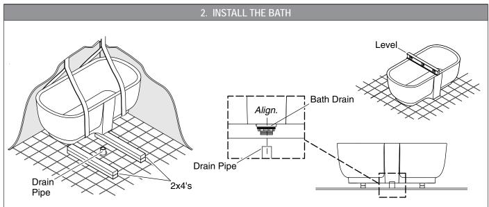
**CAUTION:** Risk of personal injury. This bath is extremely heavy. Obtain sufficient help **and** use lifting straps to carefully lift or move the bath.
