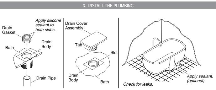
A CAUTION: Risk of property damage. Make sure a watertight seal exists on all bath drain connections.
