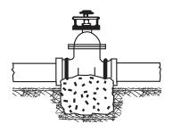
at the side of the trench. Use plywood sheets to form the block and control the pour so that the area of contact with the undisturbed trench will provide the necessary support.
