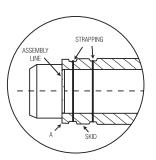
The wood used to make the skids should not be creosoted because this material will damage the pipe.
