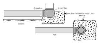
This type of hydrant foundation acts as a thrust-block, as an anchorage against frost heave and eliminates washouts from waste-water drain.
