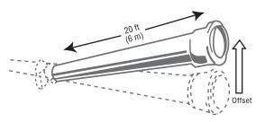
MAXIMUM RECOMMENDED OFFSETS, TO ACHIEVE MINIMUM CURVE RADIUS BY DEFLECTING A STRAIGHT LENGTH OF PIPE AT THE JOINT (FOR ALL PRODUCTS)
