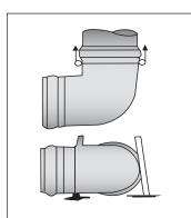
Implant 2 bars behind gasket race and grip to assemble. Bottom the pipe and pull back about 1/4" (6mm).
