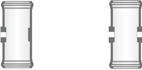
IPEX provides a simple solution for the elimination of saddles by offering PVC tapped couplings. These couplings accept standard corporation stops. For simultaneous service connections on both sides of the main, double tapped couplings are available.
