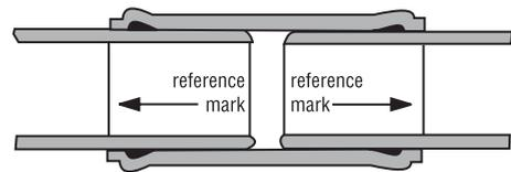
When using a section with an integral bell, more of the pipeline may have to be exposed to enable the pipeline to be deflected to allow the proper alignment of the replacement joint. When determining the length of the replacement section, take care to allow for the gap dimension on one end only. Complete the integral bell joint first then slide the double-bell coupling into place.
