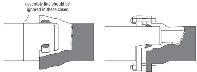
Leave a slight chamfer on CIOD PVC pipe assembled to push-fit cast iron fittings. Bottom the pipe in the iron bells.
