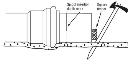
**NOTE:** *If there are no assembly lines visible on the pipe, the minimum and maximum insertion depths shown on pgs. 19, 20, 21 & 22 should be marked on the pipe by hand.*
