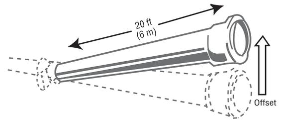
MAXIMUM RECOMMENDED OFFSETS, TO ACHIEVE MINIMUM CURVE RADIUS BY DEFLECTING A STRAIGHT LENGTH OF PIPE AT THE JOINT (FOR ALL PRODUCTS)
