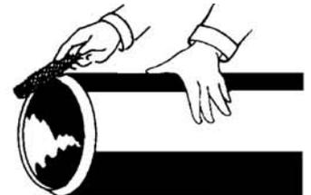
Form the chamfer using a beveling tool, hand rasp or disk cutter.
