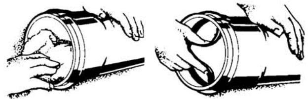
Use only IPEX PVC pipe lubricant. The use of substitute lubricants may affect water quality or damage the gaskets. For most pipes, gaskets are factory-installed.
