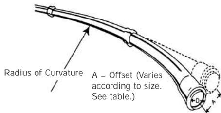
MAXIMUM RECOMMENDED OFFSET, A, TO ACHIEVE MINIMUM RADII OF CURVATURE BY BENDING THE BARREL OF 20 ft (6 m) LENGTHS
