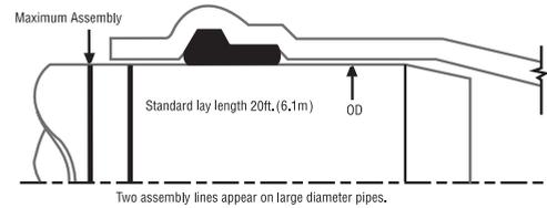
OVER-ASSEMBLY OF THE JOINT COULD DAMAGE THE BELL OF THIS OR ADJACENT PIPE LENGTHS. MAKE SURE THAT PREVIOUSLY ASSEMBLED JOINTS REMAIN UNDISTURBED.
