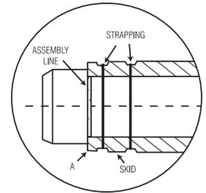
The wood used to make the skids should not be creosoted because this material will damage the pipe.
