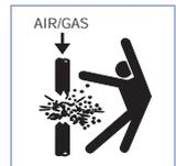
Use of compressed air or gas in IPEX municipal pipe and fittings can result in explosive failures and cause severe injury or death.
