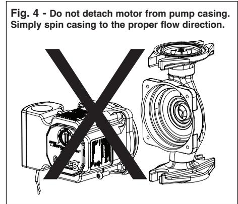
Always install with motor in horizontal orientation. Position electrical junction box at 9 o'clock for best viewing orientation. Pump casing may be rotated to change flow direction. Locate the arrow on the casing body to determine flow direction.
