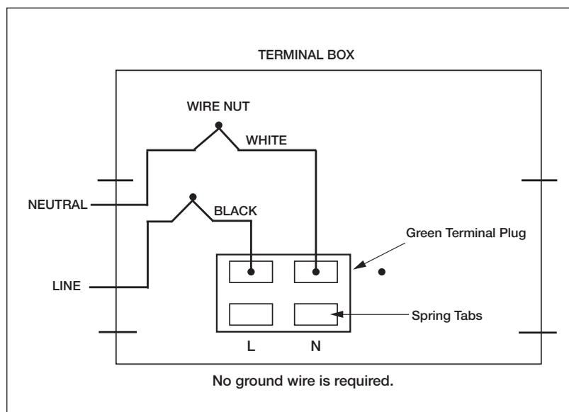
4. **Wiring the circulator:** Disconnect AC power supply. Remove terminal box cover. Attach a wiring connector into knockout hole. Use flexible conduit only. Connect Line/Hot power to the black lead, Neutral to the white lead. See wiring diagram above. The 0015e3 is a double insulated circulator; no grounding wire is necessary. Replace terminal box cover. Insert cap plug provided to cover unused knockout hole.
