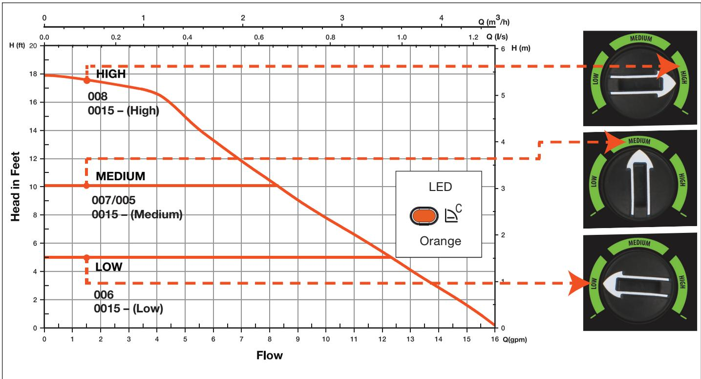
Selection options are LOW, MEDIUM or HIGH. The 0015e3 circulator varies its speed in LOW and MEDIUM setting to maintain a constant pressure differential ( $\Delta p-c$ ) in the system as heating load increases or decreases. On HIGH setting, the 0015e3 runs at full speed. See chart above for operating curves and equivalent 00 model at each setting.
