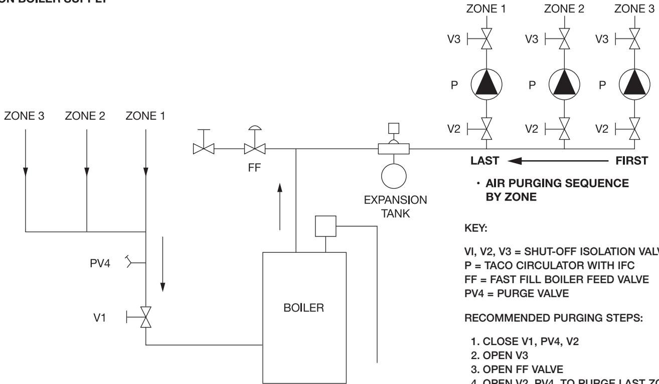
**ALTERNATE PIPING FOR CIRCULATORS ON BOILER RETURN**
