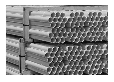
Specifications: ASTM F2158 O.D. 2.00" +.005" -.005" Wall: .060" +.005" -.005"
