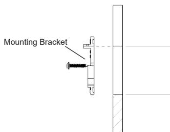
2. Align green flange so the top of sleeve hole is even with the top of drilled hole. Level the flange and mount it using the 2 screw holes provided.
