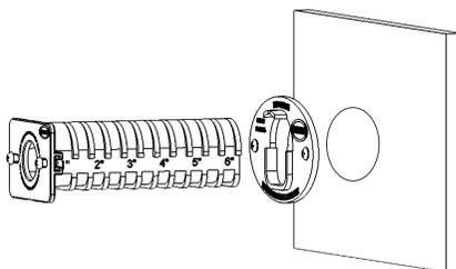
3. Insert the grey sleeve body to the desired depth, such that the outer face of the sleeve will be flush with the front of the facia (brick, stone, stucco, etc). When correct depth is set, use provided screw to lock in the sleeve through the top of the mounting flange. (Note: This screw can be removed and the sleeve adjusted at any time before the front facia material is secured.)
