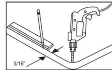
4. Using a sabre saw start cutting from the drilled hole along the cutout line. Support cutout until the cut is completed.
