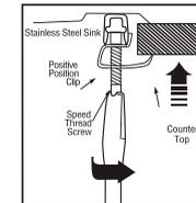
9. Rotate the clamp on the clip 90 degrees to the channel and tighten screw clockwise from the center clip using a long screwdriver.
