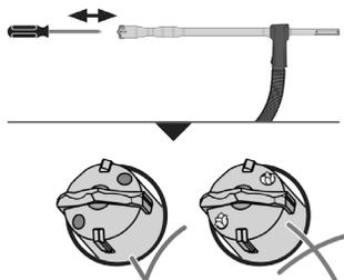
2. Ensure the bit adapter is properly attached to the bit.
