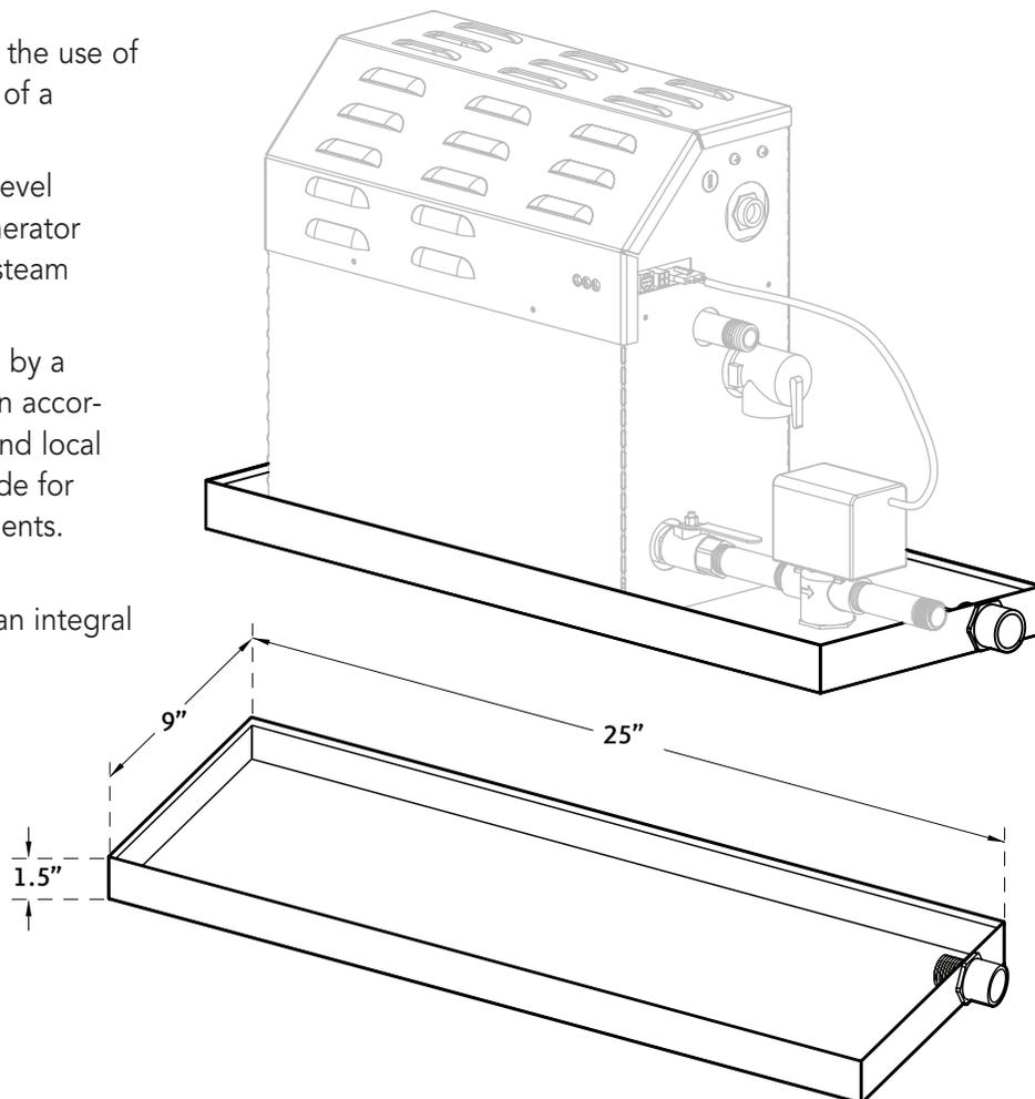
**FOR ILLUSTRATIVE PURPOSES ONLY. IMPORTANT NOTE: FOR SAFE AND TROUBLE FREE INSTALLATION** visit [mrsteam.com](http://mrsteam.com) or scan the QR code before installation to download the Installation, Operation and Maintenance Manual or refer to the manual provided with the unit.
