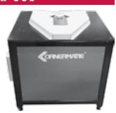
duct and corner hopper. Ductwork with acute and obtuse angles, as well as ductwork with offsets and unusual bends can easily work with the new Cornermatic+Plus machine.
