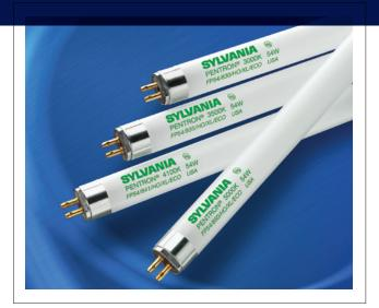
PENTRON HO XL ECOLOGIC lamps feature EXtended Life benefits of up to 60,000 hours on programmed rapid start ballasts. The life ratings reflect up to 71 percent longer life than standard T5 HO lamps, which is equivalent to an additional 3.5 years of useful life for typical operating cycles of 4,000 hours per year. The family includes 4-foot, 54 watt high output types in 3000K, 3500K, 4100K, 5000K and 6500K correlated color temperatures.
