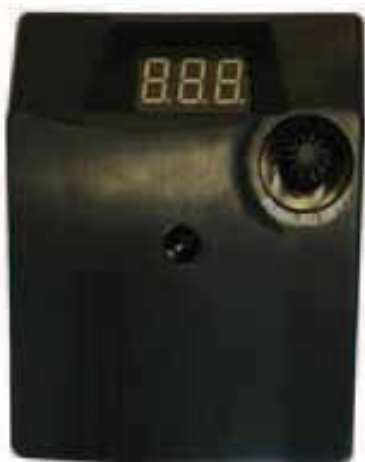
Figure 27 Water heater digital temperature control
