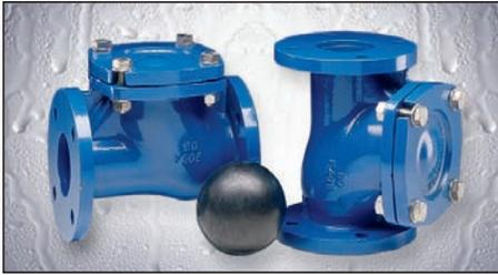
A favorite and proven valve Model in the submersible water and wastewater industry for decades. The 408 features a clean-out port permitting access to the inside of the valve without removal from the pipe line. Flanged ANSI 125 connections. Model 408FB is equipped with a "floating" rather than a "sinking" ball to prevent backflow from drains.
