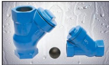
Epoxy coated Cast Iron body Model 208. Features NITRILE (Buna-N) "Sinking Ball" or Floating Ball (ad "FB" to part number). E-Z access port for cleaning or backflush. Size Range: 1 1/4" - 1 1/2" 2". Temp Max: 180°(80C)
