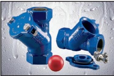
Epoxy coated Cast Iron body with corrosion resistant phenolic "Sinking Ball" (floating optional Model 508FB. Simple two bolt access cover for clean out. Feature replaceable NITRILE (Buna-N) valve seat.)
