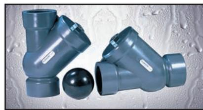
Model 208T, corrosion resistant PVC body. Threaded female x female connection. Nitrile (Buna-N) seal. Also available with PVC socket weld Model 208S. Sizes: 1", 1 1/4", 1 1/2", 2". Temp Max: 150°(65C) *Not for ground burial.*
