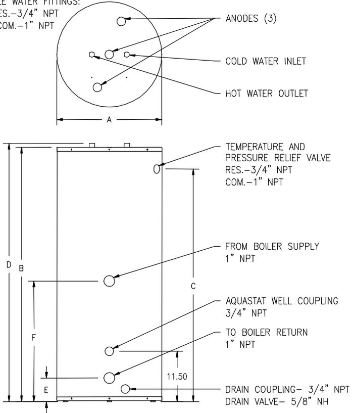
**Figure 1 – Tank Layout**
