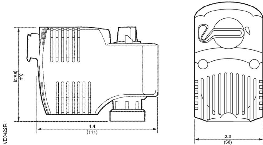
**Figure 7. Dimensions of the SFx Series Actuator.**
