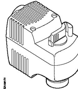
**Description** The 599 SF Series electronic zone valve actuators, accepts 24 Vac or 120 Vac power supply signal to provide two-position control. This actuator works with Siemens 599 Series zone valves with 1/10-inch (2.5 mm) stroke.
