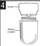
Insert light bulb into socket. Be sure to use bulb with wattage no greater than specified for this fixture. Thread diffuser into canopy.
