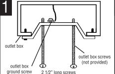
Screw green ground screw into threaded hole on cross bar between dimples. Do not tighten. Form a loop in ground wire from outlet box and ground wire from fixture. Place loops under head of ground screw and tighten. Insert outlet box screws (not provided) through oval slots in cross bar and attach to outlet box. Screw 2 1/2" long screws into the outer most threaded holes.
