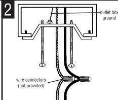
CONNECT THE WIRES. NOTE: Attach black fixture wire to black supply wire, white fixture wire to white supply wire. Do not mix them up. Use approved wire connectors (not provided).
