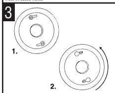
INSTALL canopy to ceiling. Push fixture wire into outlet box. Align head of mounting screws with large end of key hole slots, push canopy towards ceiling. Rotate canopy counterclockwise and tighten screws.
