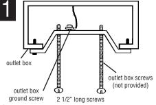
Screw green ground screw into threaded hole on cross bar between dimples. Do not tighten. Form a loop in ground wire from outlet box and ground wire from fixture. Place loops under head of ground screw and tighten. Insert outlet box screws (not provided) through oval slots in cross bar and attach to outlet box. Screw 2 1/2" long screws into the outer most threaded holes.
