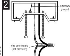
CONNECT THE WIRES. NOTE: Attach black fixture wire to black supply wire, white fixture wire to white supply wire. Do not mix them up. Use approved wire connectors (not provided)
