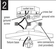
CONNECT THE WIRES. NOTE: Attach the black fixture wire(s) to black supply wire, and the white fixture wire(s) to white supply wire. Do not mix them up. Use wire connectors (not provided).
