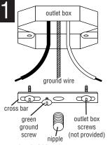
ATTACH CROSS BAR to outlet box with outlet box screws (not provided). THREAD NIPPLE into cross bar. Adjust nipple to proper height for mounting fixture
