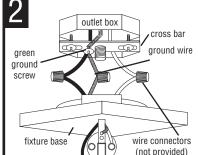
CONNECT THE WIRES. NOTE: Attach the black fixture wire(s) to black supply wire, and the white fixture wire(s) to white supply wire. Do not mix them up. Use wire connectors (not provided).
