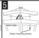
SCREW LIGHT BULB(S) INTO SOCKET. Be sure to use bulb with wattage no greater than specified for this fixture. Align holes in cage with holes in base and secure with fixture mounting screws provided.
