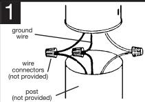
CONNECT THE WIRES. NOTE: Attach black fixture wire to black supply wire, white fixture wire to white supply wire. Do not mix them up. Use approved wire connectors (not provided). Connect bare fixture ground wire to ground wire from outlet box. NEVER CONNECT GROUND WIRE TO BLACK OR WHITE POWER SUPPLY WIRES.
