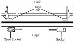
ATTACH FIXTURE ROOF TO FIXTURE CAGE. Slip one hinge pin on roof into hole in socket on cage and snap other hinge pin into open socket.
