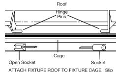
one hinge pin on roof into hole in socket on cage and snap other hinge pin into open socket.
