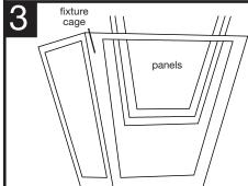
BEFORE SNAPPING HOUSING SHUT, install plastic panels, textured or beveled side out, by sliding panels down cage in slots on inside of cage. Make sure panels are all the way down into seats in cage. Some panels may fit tighter than others and a moderate amount of force may be required to install.
