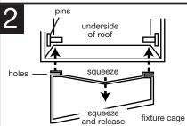
ATTACH FIXTURE ROOF TO FIXTURE CAGE. Squeeze cage as shown. Position holes on side of cage over corresponding pins on underside of roof. Release cage - pins will snap into position.
