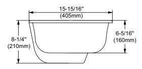
Note: All dimensions and specifications are nominal and may vary: Dimensions of  $8^{"}$  and greater have a tolerances of +3%. Dimensions less than  $8^{"}$  have a tolerances of +5%.
