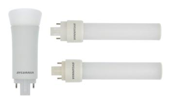
SubstiTUBE DULUX LED Pin Base lamps are direct replacements for compact fluorescent lamps. They can be directly installed without the need to bypass the existing CFL ballast. The lamps are available in GX23 and G24Q/GX24Q bases and in magnetic or electronic ballast configurations.
