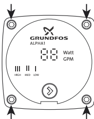
Fig. 4 Remove the four socket head cap screws on the power head to change the power head position
