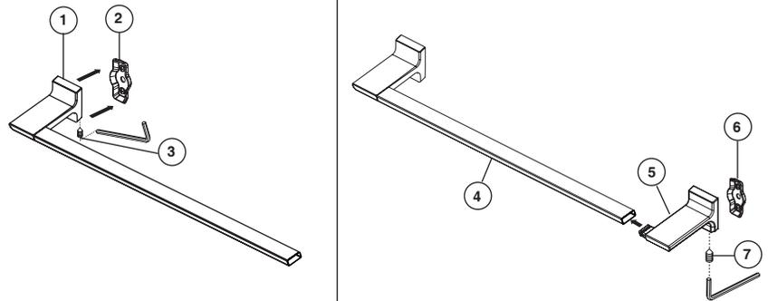
Position body (1) over mounting bracket (2) and tighten set screw (3). (Set screw should be on the bottom of body.) Place one end of the towel bar (4) into the second body (5), and place the other end of the bar into the first body (1). Slide the second body over the other mounting bracket (6) and tighten set screw (7).
