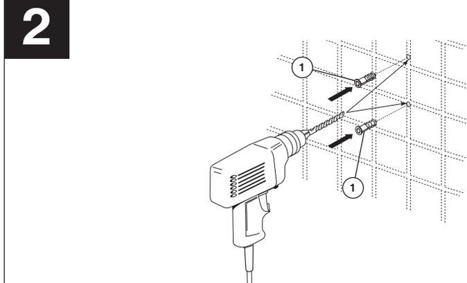
**NOTE: If possible, it is best to mount at least one end of your towel bar into a wall stud. Try to locate a wall stud with a stud finder or by tapping on the wall. Place mounting bracket (1) in the desired location. Ensure the mounting bracket is level; then, mark the position of the holes (2) on the wall. Repeat for 2nd mounting bracket, spaced as noted above.**
