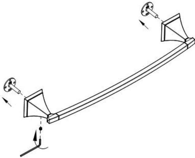
② ALIGN MOUNTING BRACKETS AND MARK LOCATION
