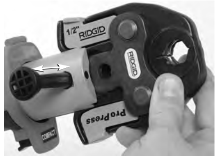
Figure 6 – Attachment Mounting Pin
