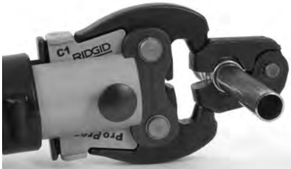
Figure 10 – Attaching Actuator to Press Ring
