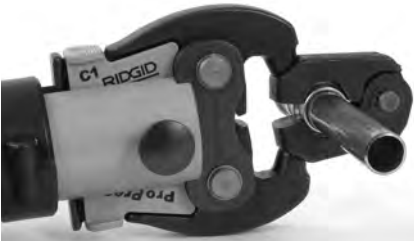
Figure 10 – Attaching Actuator to Press Ring
