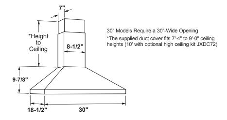
The vent hood must be installed 24" min. above the cooking surface. For optimal performance, installing the hood more than 38" above the cooking surface is not recommended. The hood installation height above the cooking surface depends upon ceiling height. The telescopic duct cover conceals the ductwork running from the top of the hood to the ceiling.
