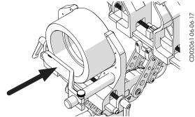
Allow insertion depth mark to protrude 3/8" to 1/2" past jaw.
