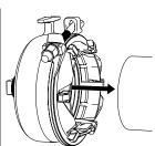
Step 4 • With the bolt in the extended position, place the end cap onto the pipe end until the pipe makes contact with the inside of the end cap. Note: If it's impossible to bottom-out the pipe, ensure there is a minimum of 4" of pipe insertion.
