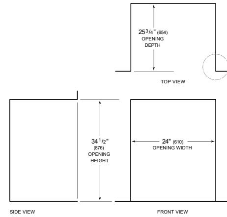
NOTE: 4 1/2" (114) finished returns will be visible and should be finished to match cabinetry.
