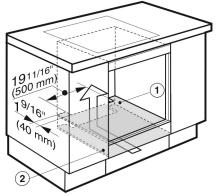
To ensure that the Combi Steam Oven has adequate ventilation, the following cut-outs measuring 19 11/16" x 1 9/16" (500 x 40 mm) must be made:
