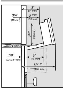
The area in front of the control panel must not be blocked by anything (such as a door handle) that would hinder it from opening and closing.
