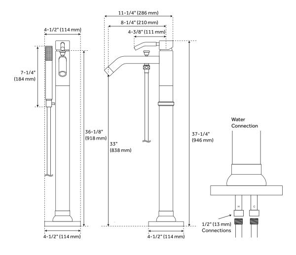
Underfloor access is required for proper installation. Installation on a concrete slab will require cutting and concrete removal.
