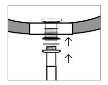
7. Thread the lock nut onto the threaded shank. Hand-tighten and make sure that the drain is properly aligned. When ready, finish tightening with a basin wrench to secure the drain
