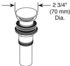
**RP81627▲** Push Button Drain less overflow holes
