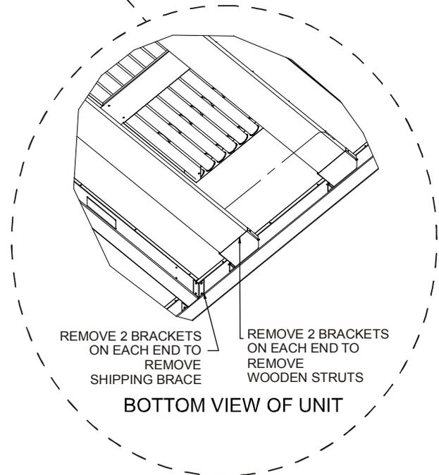
3. Lift unit per the "Rigging Details" section of this manual, observing all warnings and cautions. When unit is lifted, boards and shipping brace will drop if screws have been removed. To avoid injury, STAND CLEAR.
