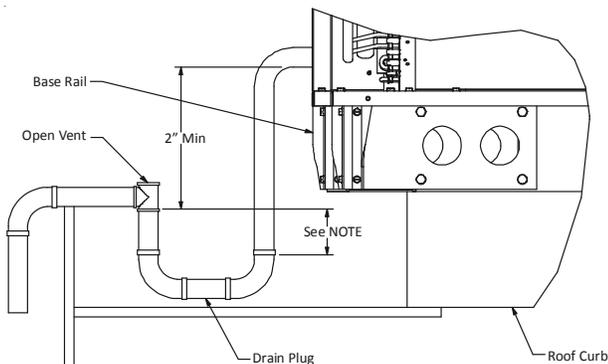
**NOTE:** Trap should be deep enough to offset maximum unit static difference. A minimum 4" trap is recommended.
