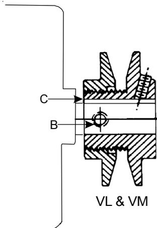
**NOTE:** Do not operate sheave with flange projecting beyond the hub end.
