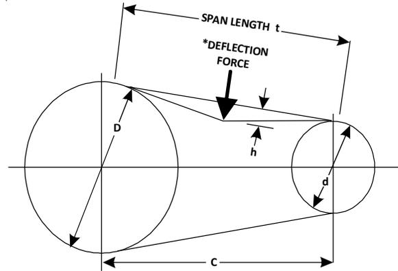
*\*Apply force to the center of the span.*
