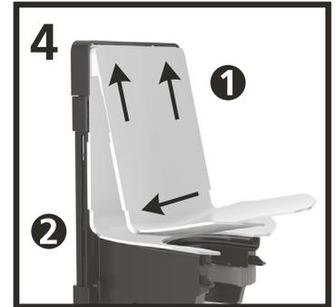
Attach the back plate by pressing on the top two corners and the bottom middle section.
