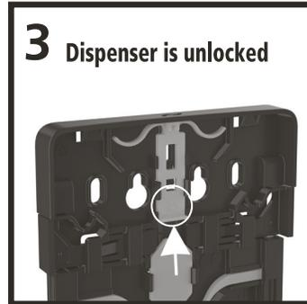
Restore to the unlocked position by pushing the locking mechanism toward the top of the dispenser.
