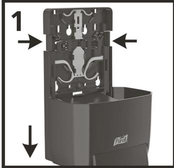
Open dispenser by pressing release buttons on side of dispenser and slide the front cover down.
