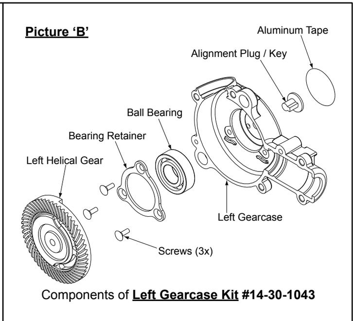
Picture "A and B" show the components that make-up the Right and Left Gearcase kits for M18™ FUEL™ Hackzell® 2719-20. Each kit contains one [1] Alignment Plug / Key and [1] round Aluminum adhesive backed disc (not sold separately) which will be needed when servicing / replacing the gearcase assemblies of the M18™ FUEL™ Hackzell®.
