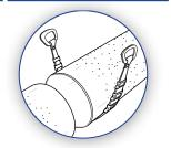
Prepare both pipe ends of the existing pipe by descaling if required. Clean the pipe using water. Make sure that the pipe is clear from debris and defects that may interfere with the HYMAX's proper seal.
