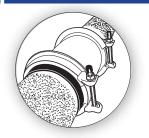
Position the coupling for installation. If possible place the couplings on the replacement pipe with top-facing bolts and lower the pipe and couplings into the ditch. Slide the couplings outward so that it covers the marks made in step 3. Make sure that the pipes are not touching inside the body of the HYMAX. There must be space between the pipes in order for continuous dynamic deflection to take place.
