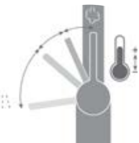
Remove the lever and turn the ring nut inside to limit the flow temperature*
