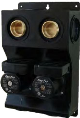
**SuperBrute XL Flow Center with two Grundfos UPS60-150 pumps in series:** The all-in-one design of the SuperBrute XL provides pumps, valves, and foam-insulated cabinet in one package. Large 2" full-flow 3-way flushing and isolation valves are designed for higher flow rates associated with light commercial and large residential applications.
