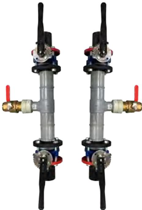
3" and 4" flushing assembly: PP-R body, HDPE fusion connections to/from ground loop and building, 2" brass ball valve flushing connections, butterfly isolation valves (sold as a set, as shown)
