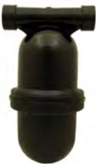
**Pressure Battery:** The industry's first polyethylene fusion expansion tank maintains system pressure via a custom-molded internal rubber bladder. The completely sealed tank never needs maintenance, and may be installed in the mechanical room, or even buried outside with the ground loop. Designed for up to 6 tons (approx. 3/4 gallon).
