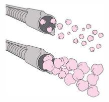
Different density settings when in attic mode to ensure tight attic spaces are adequately and easily insulated.
