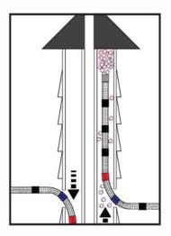
A unique wall-blowing mode with a special hose attachment makes reinsulating walls easy, quick and only requires one insertion hole.
