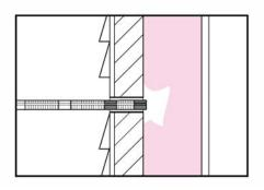
5. Feed hose down into the wall cavity until the hose is just below the top of the outlet height. This ensures insulation fills below wires crossing the cavity.
