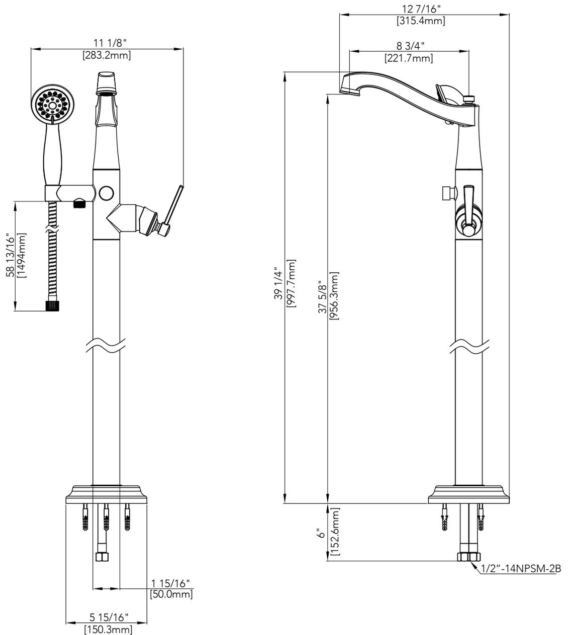
**\*\*\*Remote thermostatic valve may be needed; verify local code requirements.**
