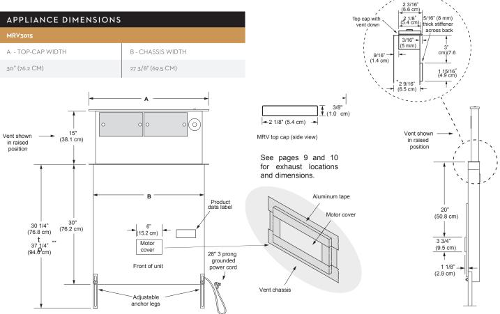
\* Total chassis depth with optional CABP3 blower installed is 10 3/8" (26.3 cm).
