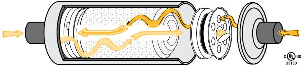
The BF Series bi-flow filter-drier is designed specifically for heat pump or a reverse cycle application. External check valves are not required since they are incorporated within the filter-drier.
