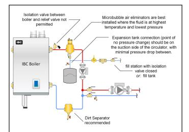
In the case of hard water, use distilled or purified water. Glycol systems require the use of propylene glycol. For large volume systems, the optimum hardness is  $\leq 2$  grains.
