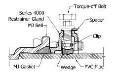
Hand tighten the Torque-limiting twist-off bolts
