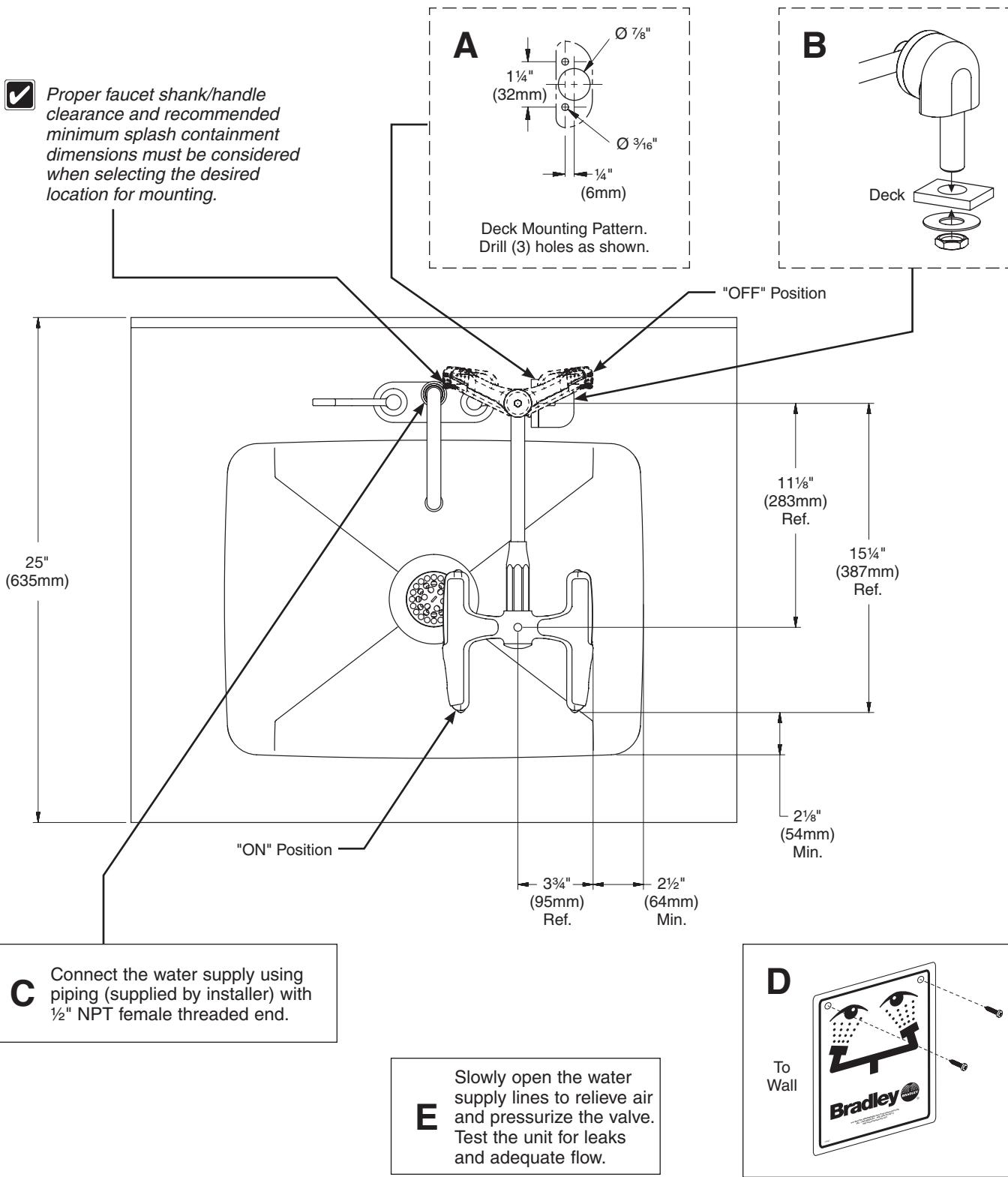
**Assembly of Components — S19-270HD, S19-270HW**
