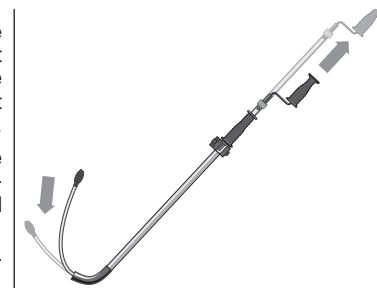
Figure 5 – Retracting the Cable
