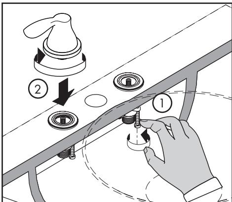
Tighten the tensioning screws.
