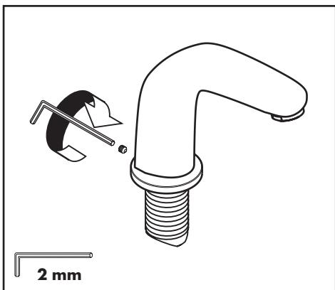
If necessary, tighten the spout screw.
