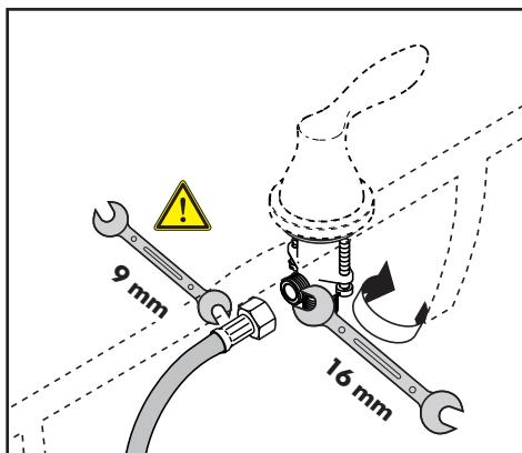
Connect the hoses to the valve outlets.
