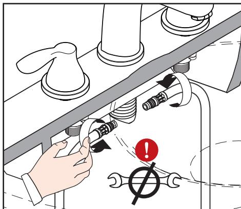
Screw the connecting hoses into the spout tee.
