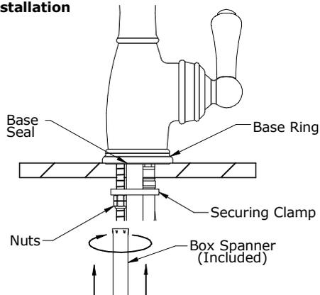
Before installing the product, leave a gap of 1 1/2" minimum from the center of the work surface hole to any walls or shelves (see image in section 5).
