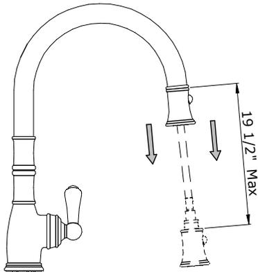
Ensure there is ample room in the space under the work surface for the hoses and weight to move freely. Test that the spray head extends far enough by pulling it out.
