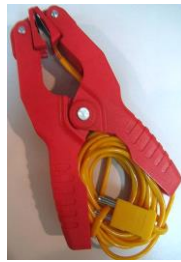
MA-12355B CLAMP-ON PROBE K-TYPE THERMOMETER JAW OPENING 1-3/8" TEMP: -40F TO 392F (-40C TO 200C) 10' LEAD
